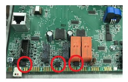
Figure 2. New-Style shunts
