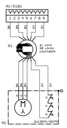
35,2 ohms between 2 motorwires at cold motor ca. +15...+30°C (+59°F...+86°F)
