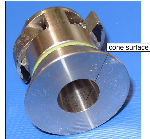
picture 4 clean surface without scratches / Darstellung saubere Konus fläche
