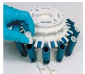
12-place rotor with removable inserts
