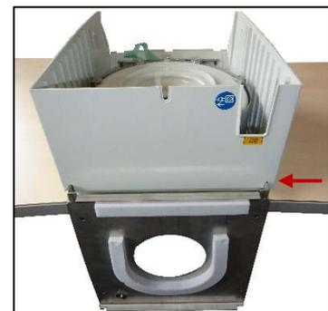
**Leave the screwdriver inserted to prevent the lid from falling down.**
