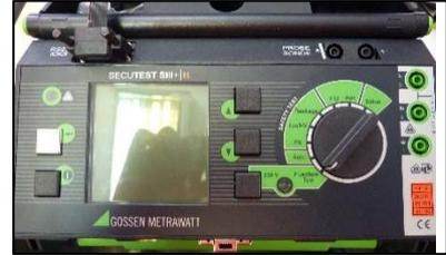
Record the measured values in the safety test section of the calibration form. Determine whether the values recorded meet the specifications on the form. If the specifications are met, this test is finished. If the specifications are not met, check for missing grounding connections and / or faulty parts.
